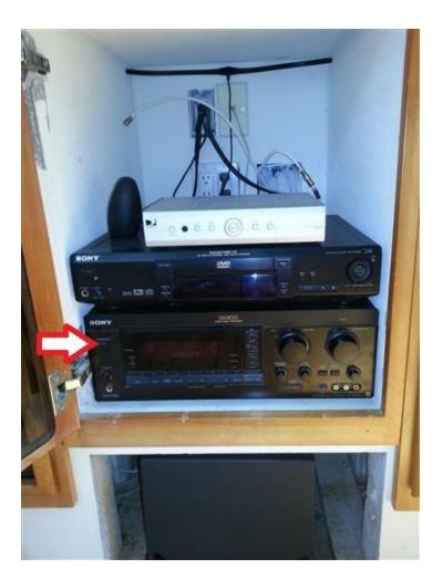
Use the large knob on the right of the SONY receiver to adjust the volume. Use the large knob on the left of the SONY receiver to change from SATELLITE to DVD, if you want to play a DVD. It should say "SATELLITE" for the Direct TV to work.
